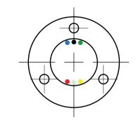
Number of rings: 6 rings Rated voltage: 0-240VAC/VDC Rated current: 2A/ring Dielectric strength: 500VAC@50Hz,60s >500MΩ/500VDC Insulation resistance: <0.01Ω Dynamic contact resistance: Contact material: Precious metals Housing material: Engineering plastic Operating temperature: -20°C≈ +80°C 0≈ 250 rpm Operating speed:
